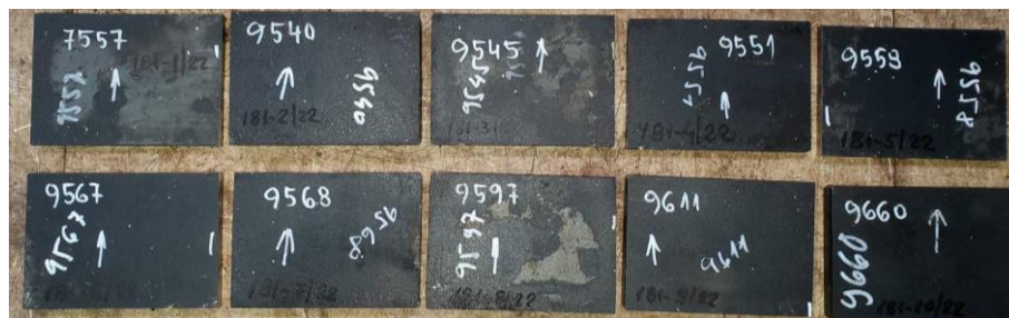
Figure 2. Test plates from which specimens for impact toughness and grain size testing were taken
