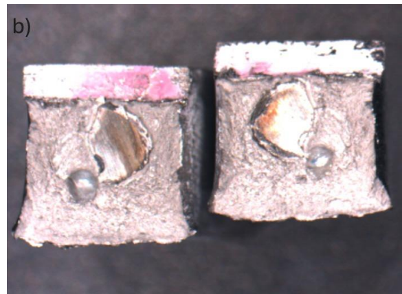
Figure 4. The surface fracture of the No1 sample: a) with a notch in the HAZ and b) with a notch in the WM, 6.3x
