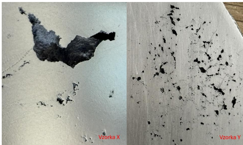
Figure 8. Visible differences in porosity on the examined samples
