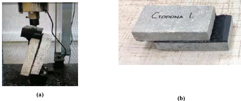
Fig. 4. Testing of a layer of sprayed waterproofing with double-sided adhesion, laid between two wall structures, for shear resistance: (a) Sample during shear tests; (b) Sample after testing.
