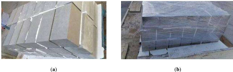
Fig. 2. (a, b) Samples processed to target dimensions 30x15x15 cm.
