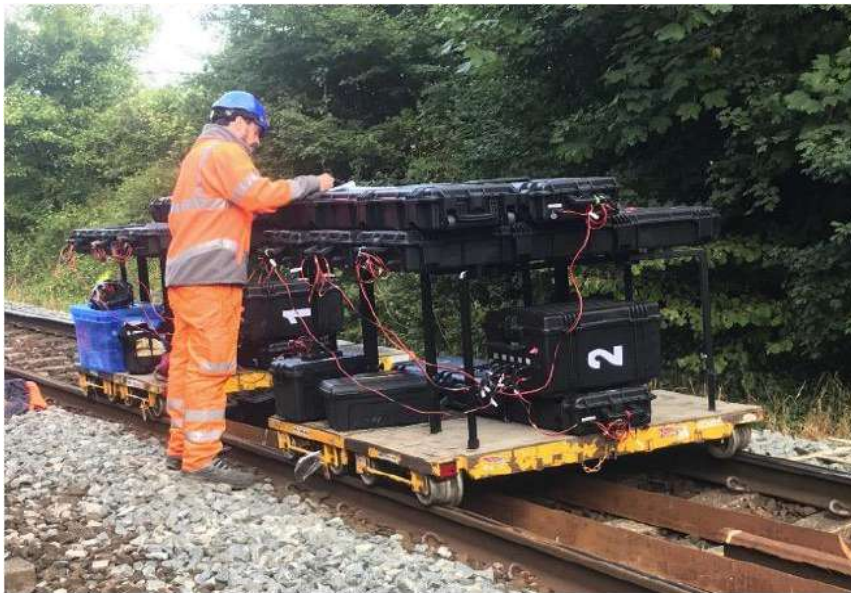
Fig. 1. Image of two planar muon systems deployed on railway tracks.
