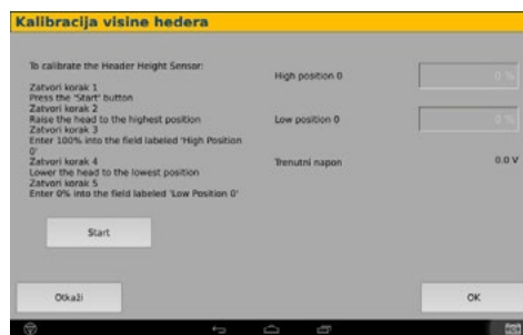
Figure 13. Header height calibration
