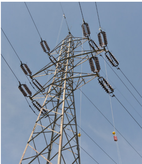
Figure 3. The probes for electric and magnetic fields attached to the phase conductors
