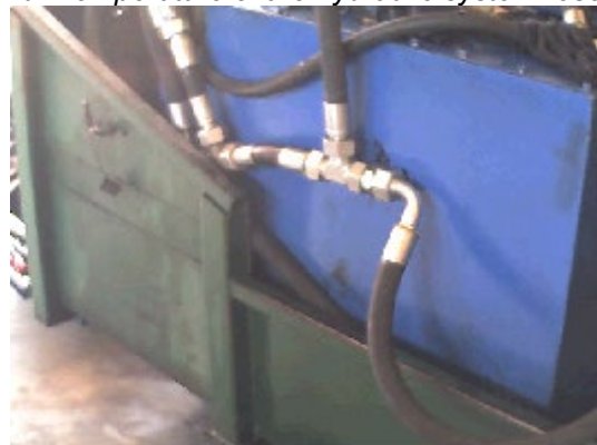
Fig 4b. Hydraulic reservoir.
