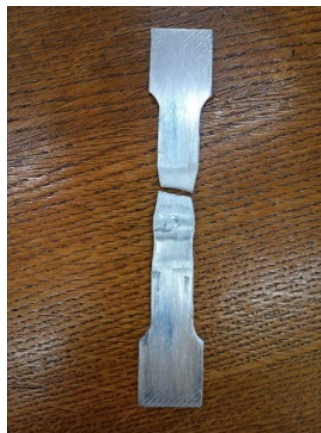
Fig. 2. The fractured specimen after tensile testing
