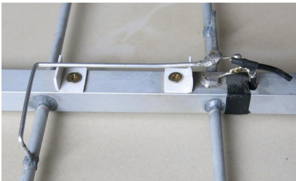
Fig. 9. A detailed view of the plastic spacers, feeding points and compensation of the reactive part of the antenna's wave impedance using pieces of coaxial cable
