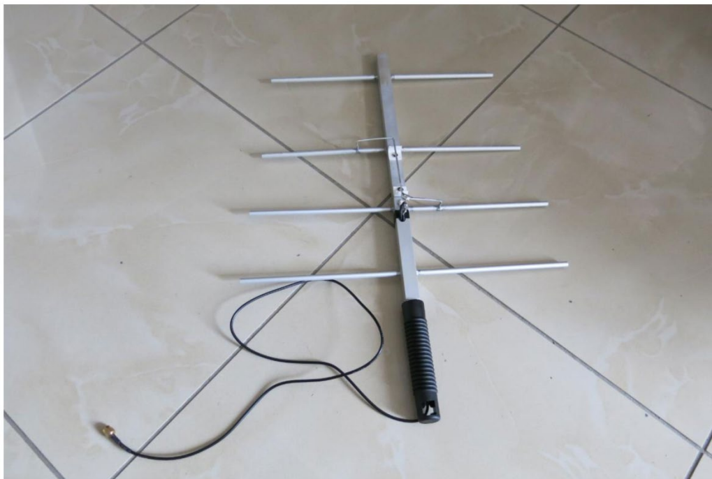
Fig. 8. Handheld HB9CV antenna with four elements (two active elements and two parasitic elements). The antenna was assembled by the authors
