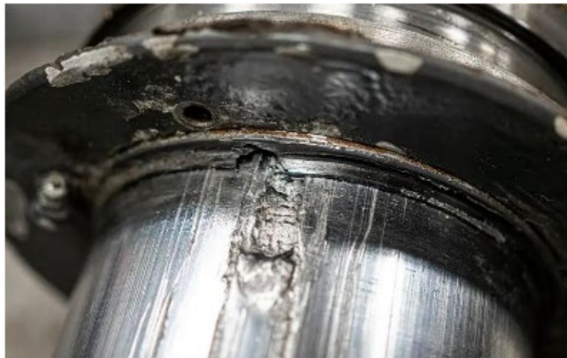
Fig. 1. Cylinder piston rod exposed to the wear process[7].
