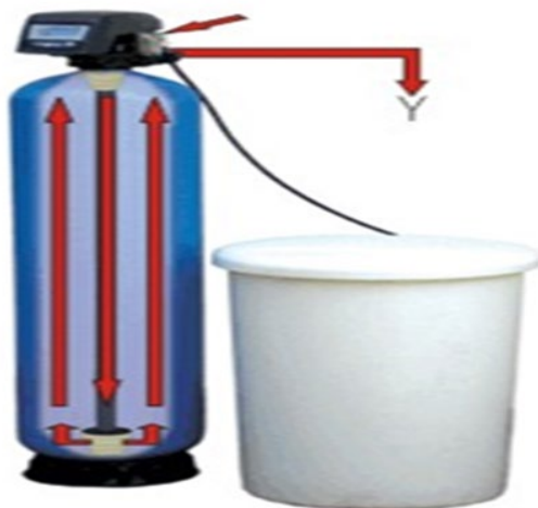
Fig. 4. Countercurrent rinsing phase
