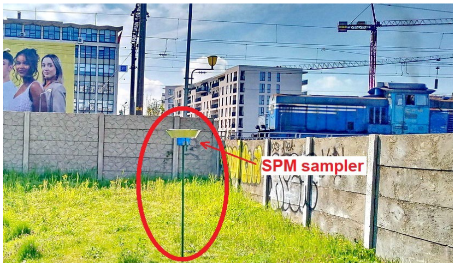
Fig. 3. SPM sampler in Timisoara, at INCUBOXX site with industry, rail & road traffic sources.
