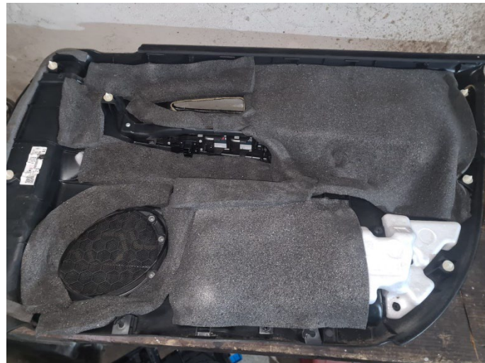
Fig. 6. Front door plastic cover with STP Biplast 15
