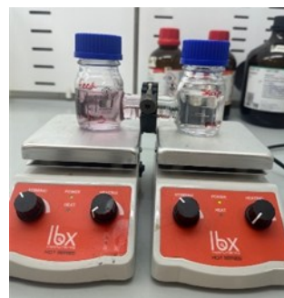
Figure 2. Laboratory extraction system based on PIM.
