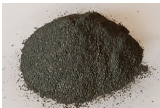
Figure 1. TiAl6Nb7 titanium powder after grinding of the hydrated sample [1]
