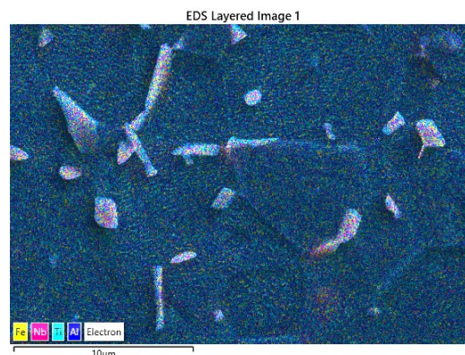
Figure 2. EDS representation of the primary phase of the matrix and the secondary phase [2]
