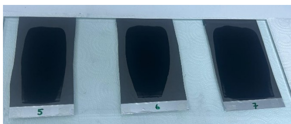
Figure 1. Cathode electrode coated via slurry-casting method.
