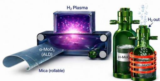
Figure 1. Concept of rollable solid-state hydrogen storage device.
