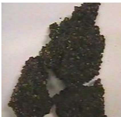
Figure 2 Sinter with 70 % concentrate and 30 % catalyst
