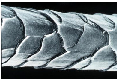
Figure 1. Electron micrograph of a clean Merino wool fiber showing overlapping cuticle scales. The scale structure contributes to the directional friction central to wet felting. Source: CSIRO ScienceImage 2487 (2000), CC BY 3.0; cropped [6].
