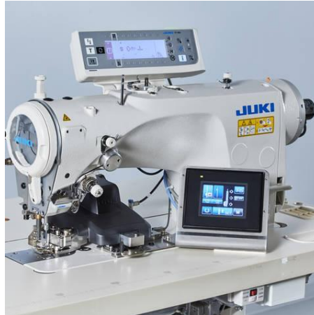
Figure 12: JUKI sewing machine for sewing “AiryString™” tapeless zippers
