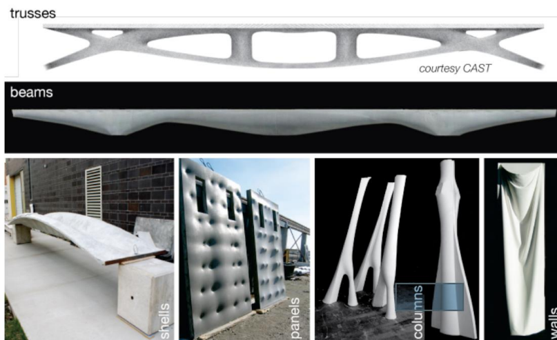
Figure 1: Research into various applications of textile formwork (Mark West (CAST), according to [22])
